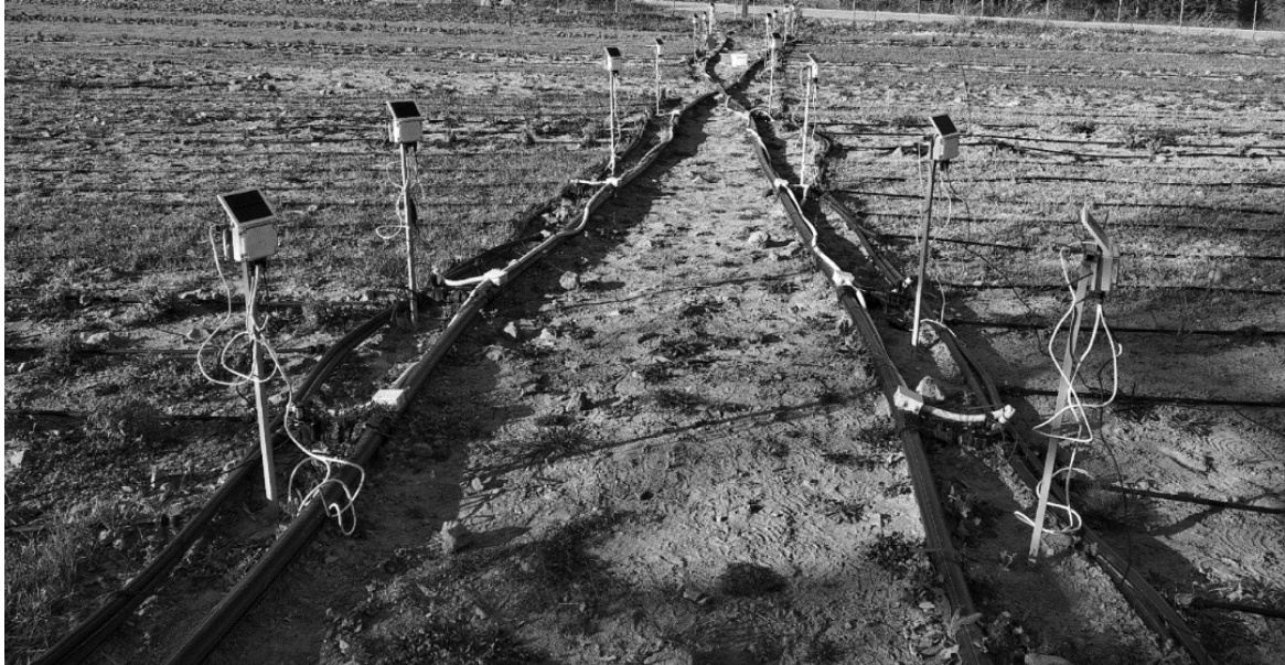
Fig. 1 The wireless sensors (WS) placed in the experimental site
