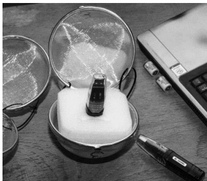
Fig. 4 Insertion of a data logger into a protective sieve
