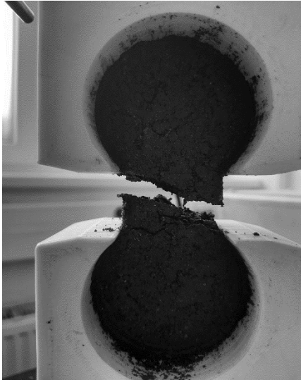
Fig. 3 Tensile test of simulated (a and b) and measured (c) samples. Adhesive force distribution in soil sample before rupture (a) and after that (b) with fracture line.
