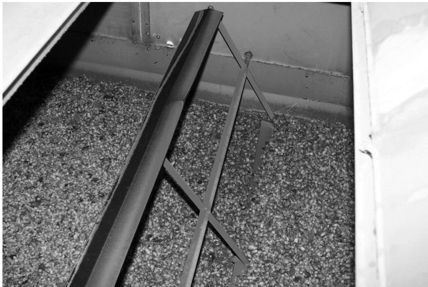
Fig. 2 Rotor between the first and second inspection window above the first belt of the belt dryer
