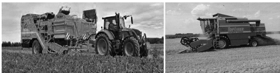
Fig. 1 Agricultural machines previously produced were constructed mainly of classic materials (iron, steel, aluminum, various metal alloys). Their weight was therefore significantly greater than the current machines. The two-row potato harvester is shown on the left, the grain harvester on the right.
