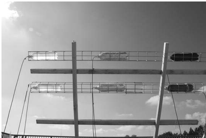
Fig. 1 Six variations of sterilisation bottles exposed to the sun.
