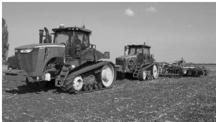
Fig. 1 Photo of draft measurement of chisel plough Horsch Tiger 5 AS at Sloveč in autumn 2018.
