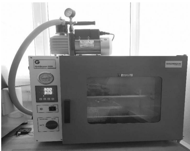
Fig 3: Goldbrunn I450 vacuum dryer for vacuum drying.
