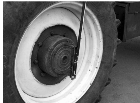
Fig. 3 Tractor's wheel with sensor-hermetic contact
