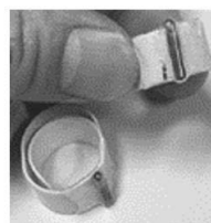
Fig 9. Mounted the RFID tag with a heat-shrinkable tube for leg ring
