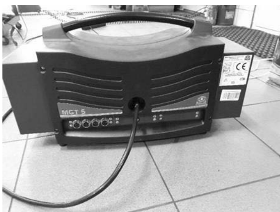
Fig. 4 MGT-5 exhaust gas analyzer
