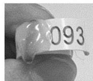
Fig 6. The RFID tag mounting for chicken leg ring with a hot melt adhesive (ethylene vinyl acetate)
