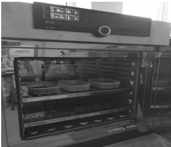
Fig 2: Memmert UF110 convective dryer for normal drying.
