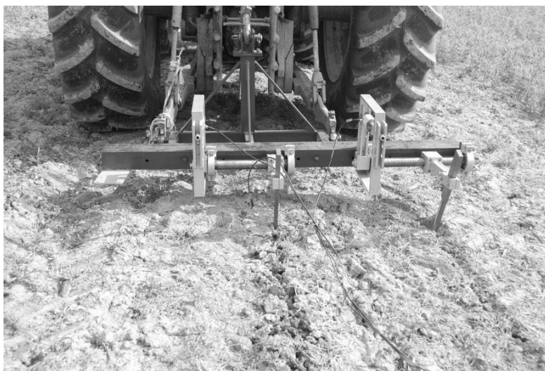
Fig. 1 Horizontal penetrometer using h the two-argument comparative method - photograph from the measurement
