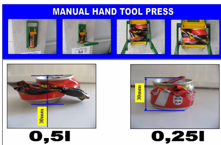
Figure 3 Hand tool manual pressing of ALU cans 0.25 liters and 0.5 liters
