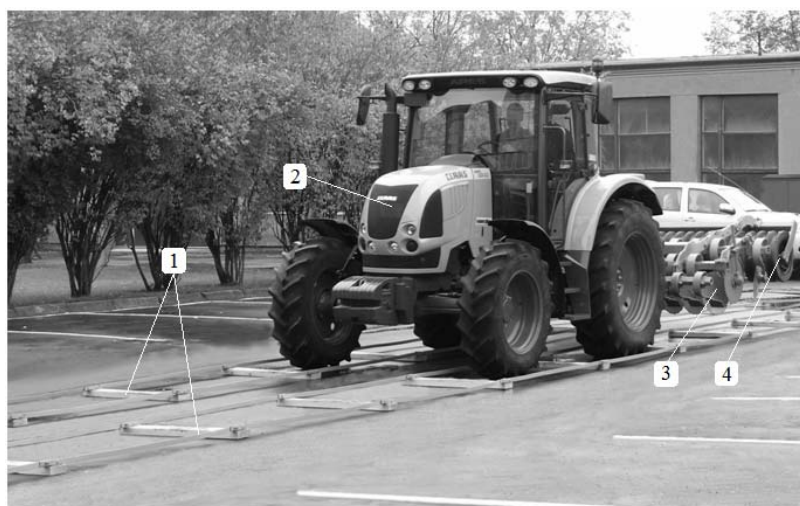
Fig. 1. Tractor Claas Area ATX 557 movement over artificial roughness test road 1 – Artificial roughness test road; 2 – Tractor Claas Ares ATX 557; 3 – LEMKEN short disk harrow; 4 – LEMKEN rubber rings roller.
