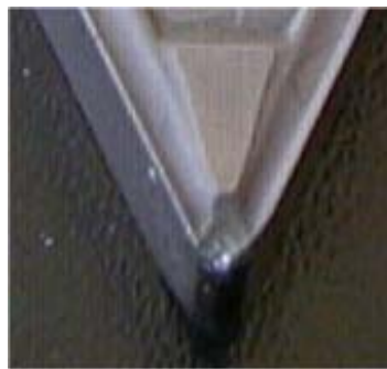
Fig. 5 Worn cutting blade after turning of the specimen No. 2
