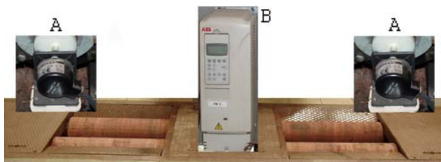
Figure 1 Roll test bed: A - Incremental sensor of roller's revolution, B - Frequency converter
