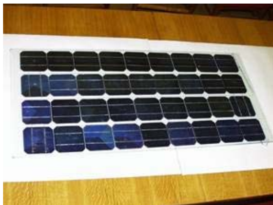
Fig. 1. Photoelectric solar module with organic-silicon polymeric materials (manufactured at the VIESH). Dimensions: 450 × 970 mm; electric power: 50 W; voltage: 12 V
