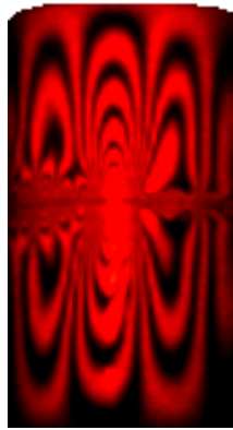
Figure 02. Stress distribution in cans with diametrical compression loading. (Crespo, 2006)
