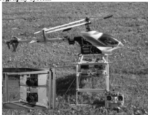
Figure 2. Aerial photography system with the hobby-use radio controlled helicopter
