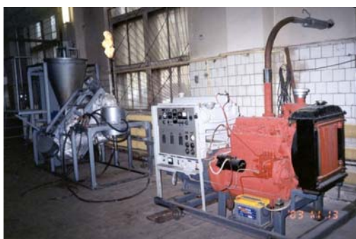
Fig. 11. General view of the installation for obtaining fluid and gaseous biofuel with a productivity of 0.5 tons per day, developed in VIESH by M.V. Yerkhov, and a diesel generator, 30 kW in power (on the right), fed with the biofuel.
