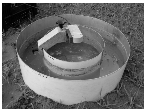
Fig. 1: Double rings infiltrometer Eijkelkamp with telemetric ultrasonic sensor
