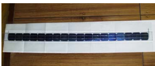
Fig. 2. Double-sided photovoltaic receiver, intended for a stationary concentrator (designed at the VIESH).
