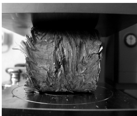
Fig. 5. Straw briquette in the ZWICK testing equipment.
