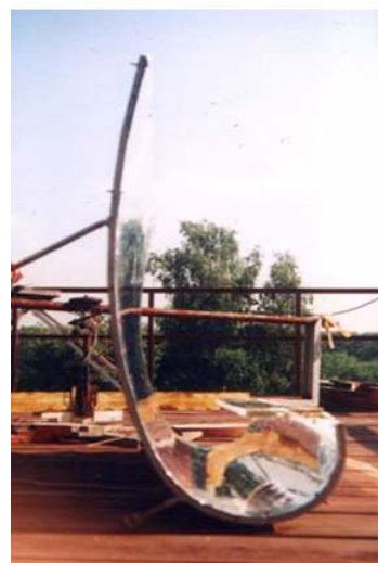
Fig. 4. a – Solar facade with an asymmetric vertical solar module, having an aperture angle of 48^\circ : 1 – glass cover; 2 – reflector; 3 – aperture angle; 4 – double-sided photovoltaic receiver; 5 – southern facade of the building b – Photo of an experimental module with a solar concentrator
