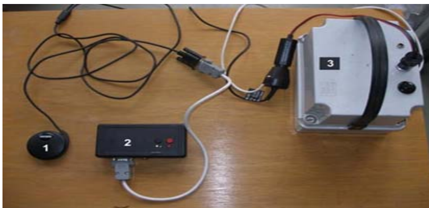
Fig. 2. Equipment for data collection, 1 – DGPS receiver, 2 - data storage unit, 3 - battery.
