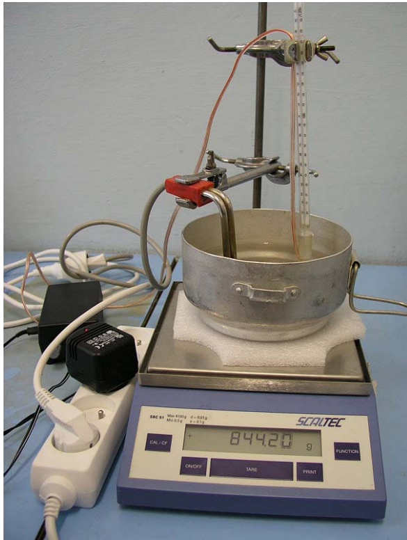
Fig.6 The experiment for measuring of evaporation speed
