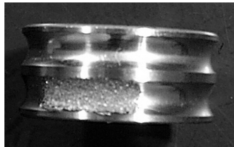
Fig. 1. Example of a extended fault in the inner race.
