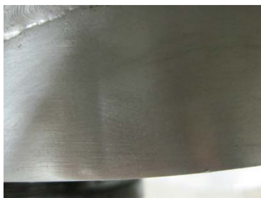
Fig. 6 External surface of fermentation tank after cleaning
