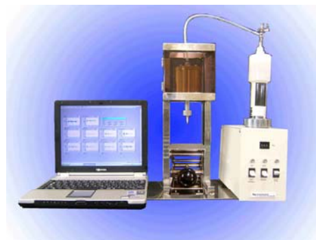
Fig. 3 Photograph of AMC system for measurement of texture index.
