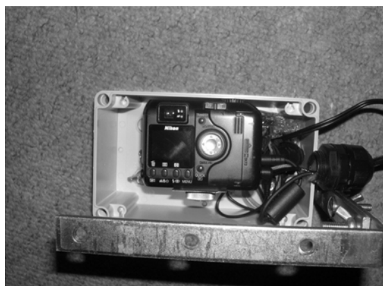
Fig.3. Camera fixed inside plastic box by help of tripod screw.
