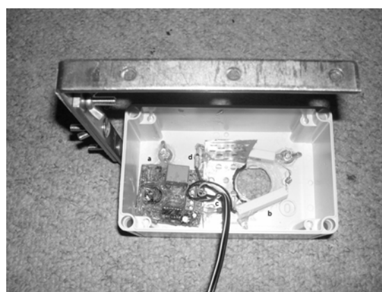
Fig.2. Opened plastic box prepared for camera instalation. a-thermostat, b-10Ω resistors, c-temperature sensor, d-temperature protection.
