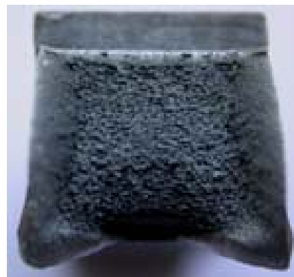
Figure 5 Ductile fracture of steel 21MnTiB at the temperature 20 °C
