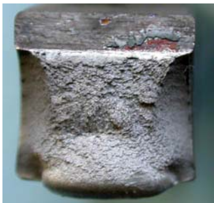
Figure 6 Fracture area of steel 21MnTiB at the temperature -40 °C. Semi-brittle fracture.
