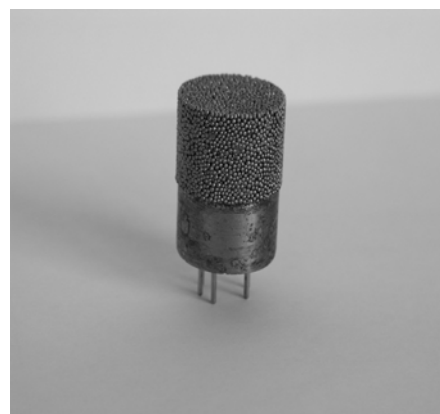
Fig. 2. The case of sensor – sintered metal housing. Diameter is 15 mm.
