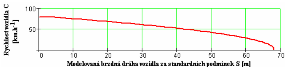
Figure. 3 - Braking distance of measured vehicle Škoda Octavia 1.9 TDI
