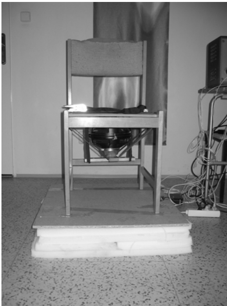
Fig.2. Special constructed vibration seat.
