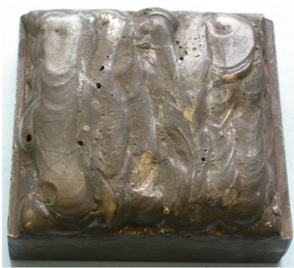
Figure 2 Overlay using the electrode 65 – 3
