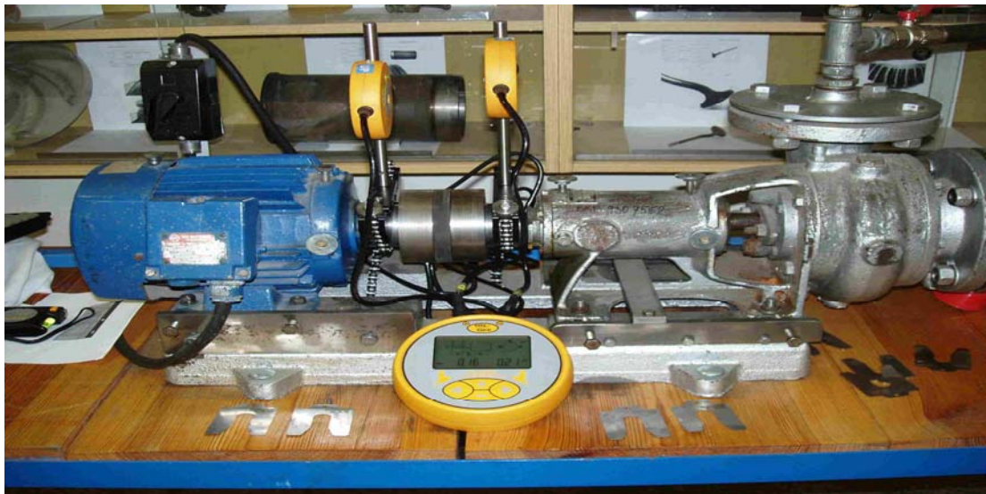
Figure 1 - Experimental set up for the shaft connection with the Fixtur laser Colibri.
