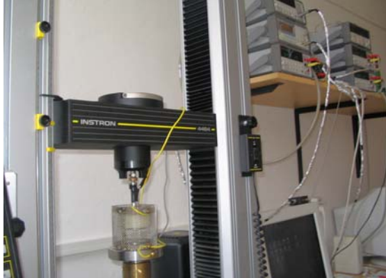
Fig. 2 The electric equipment for measurement of dielectric properties of the specimen during its mechanical testing. The testing machine Instron is in the left part of the photo with the tested specimen fixed below loading cell. In the right upper part, there is electric part of the equipment.
