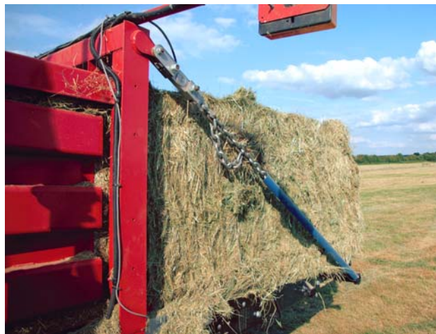
Figure 2. Proprietary tension dynamometer fitted to the chains supporting the bale chute. After: Maguire et al, (2007)
