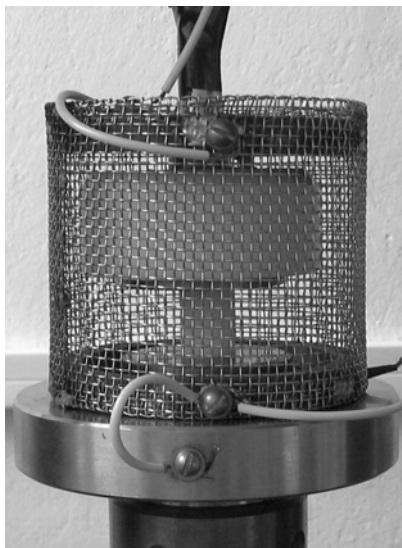
Fig. 3. Specimen arrangement in testing machine: between two metallic plates in Faraday cage.
