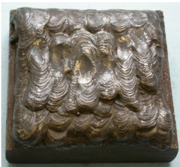
Figure 4 Overlay using the electrode 650 – 3
