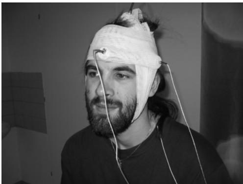
Fig.3. Accelerometers connected on the head of passenger in three main axis of body.
