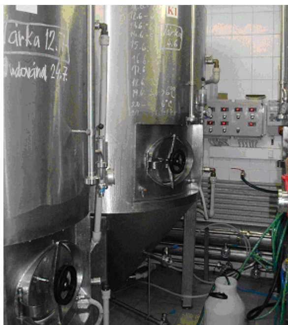
figure 2 – fermentation tanks (Tutorial and Research Brewery of the University of Life Science Prague)
