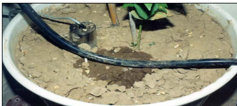
Figure 3 - Soil moisture sensor Virrib under laboratory conditions
