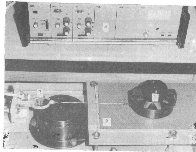
FIG.1: The detail of the working part of the tribometer 1. testing body - 2. sliding plate - 3. tensometric sensor - 4. tensometric apparatus
